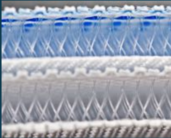
View of a 2-layer 3D Spacer Fabric
